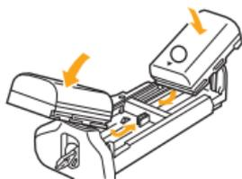
2. **Canon LP-E6 Batteries:** Insert up to two batteries by placing them in either slot in the battery tray, ensuring the correct orientation as shown on the tray.
