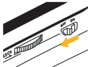
5. Switch the grip power to ON and then turn on the camera's power. Check the battery level in the control panel or viewfinder.
