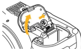
3. Open the camera battery chamber cover and remove, as indicated above.
