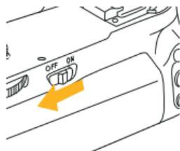
1. Ensure that the power is turned off on the camera and that the power switch is set to OFF on the battery grip.
