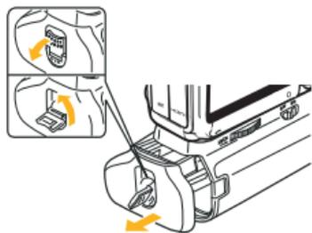
1. Ensure that the power is turned off on the camera and grip. Use your fingernail to pry open the battery tray lever so you can rotate and pull it as indicated above and slide the battery tray out of the grip.
