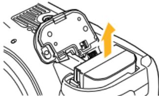
2. Remove the battery from the camera battery compartment.
