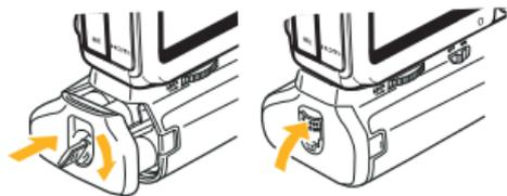
4. Rotate the battery tray lever counterclockwise and slide the battery tray all the way into the grip. Rotate the lever as indicated above and push it back into place to lock the tray.
