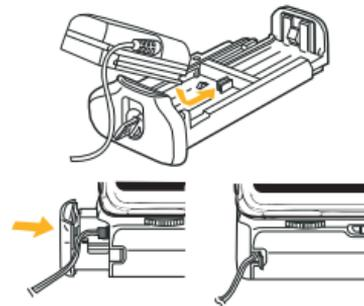
6. **Household Power Outlet:** The Canon ACK-E6 AC Power Adapter Kit (sold separately) can be connected to the grip. Insert the DC coupler through the small groove on the back of the grip. Ensure that the cord doesn't get pinched by the battery holder.
