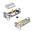
3. Nikon EN-EL15 Battery: Line up the indentations on the battery with the EN-EL15 holder, then press the battery down and slide it in the direction of the arrow until the power terminals click into place.
