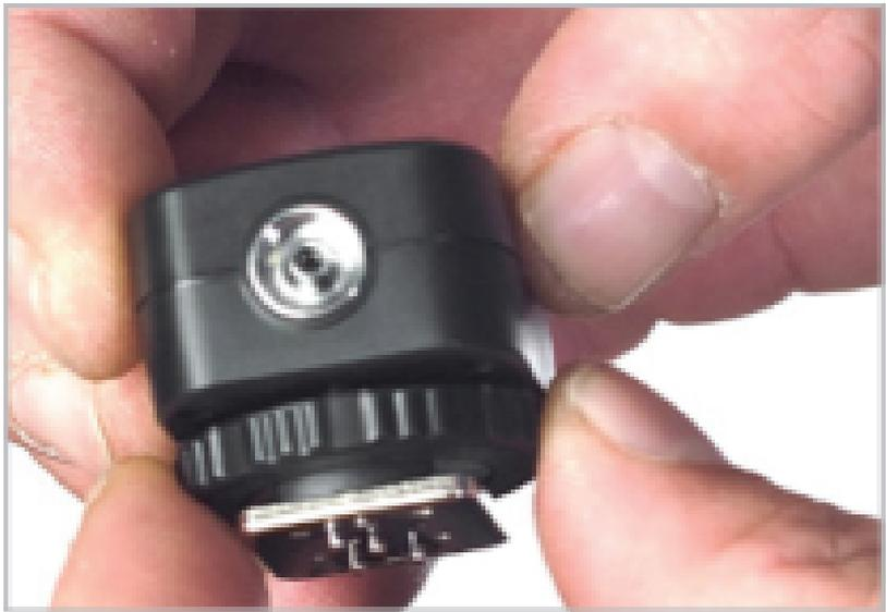
2. Insert the adapter's hot shoe into the camera's hot shoe mount.
