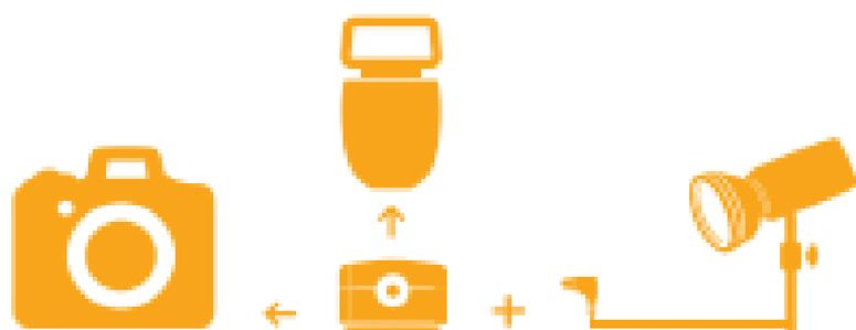
The PSU model is a universal adapter with a PC sync terminal and a top hot shoe that allows you to have a flash mounted on the camera while simultaneously connecting the camera to a studio light via a PC sync cord. This adapter does not offer TTL metering.
