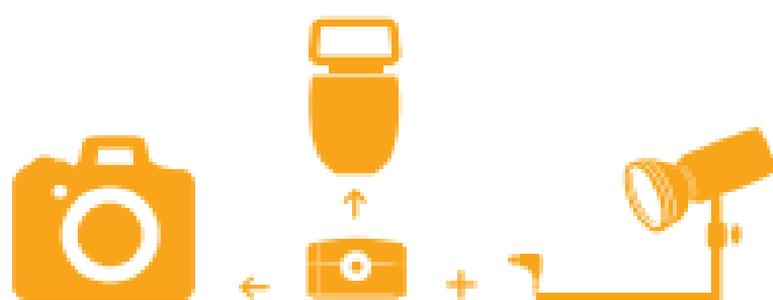
Models PSC, PSS, and PSN allow you to have a flash mounted on the camera while simultaneously connecting the camera to a studio light via a PC sync cord. The adapter's top hot shoe offers full TTL metering for the specified camera.
