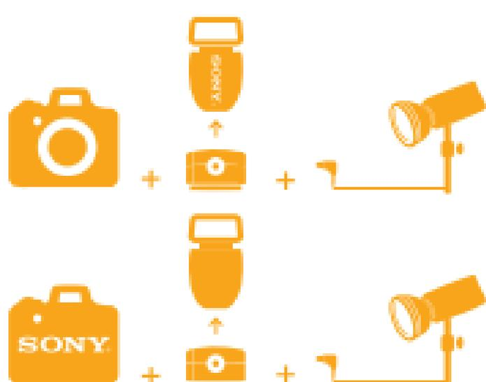
Model CSC allows you to use universal flashguns on Sony and Konica Minolta cameras. Model CCS allows you to use Sony and Konica Minolta flashes on non-Sony or Konica Minolta cameras. The converter also incorporates a PC sync terminal, enabling you to simultaneously connect your camera to a studio light via a PC sync cord. These models do not offer TTL support.
