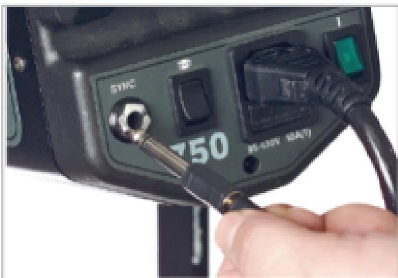
**Warning: Not to be used with older flash units having a trigger voltage of more than 6v.**
