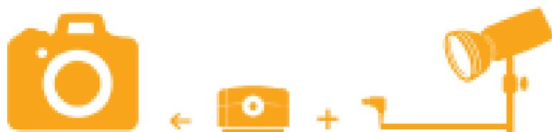
Models PCU and PCS add a PC sync terminal to your camera, allowing you to connect a flash sync cord fitted with a standard PC type connector via the camera's built in hot shoe.
