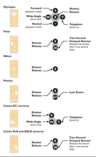
**Note:** The 2S button will start shooting video on compatible Canon DSLR cameras when in video mode, the T and W buttons will not work with Olympus E-system cameras, and the W/T button will not work with Pentax SLR and DSLR cameras. Specific functions may vary depending on your camera.
