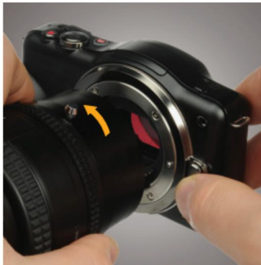
2. Rotate the lens assembly counterclockwise to release.
