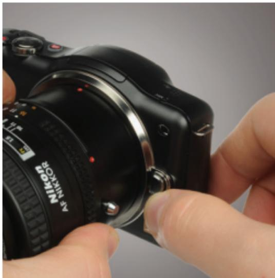
1. Press the lens release button on the camera.
