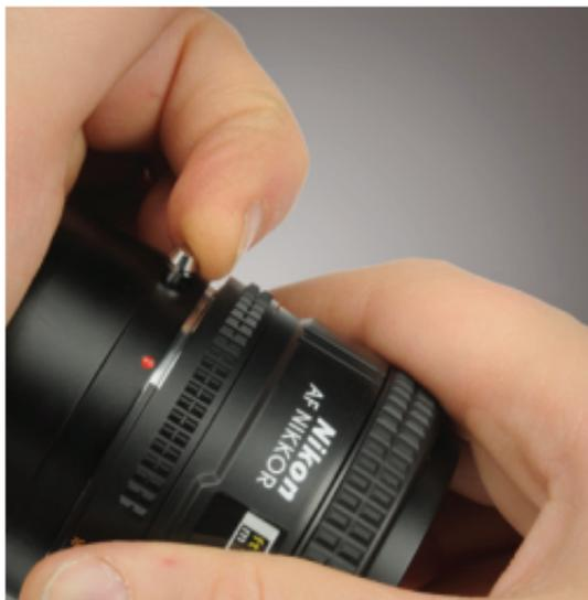
**3.** Lift and hold the release pin on the lens adapter.
