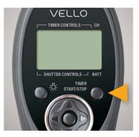
Once you've set up your Timer Controls, press the Timer Start/Stop button to begin the countdowns and exposures.
