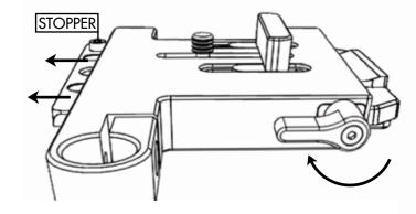
Push BASE until contact is made with STOPPER before tightening thumbscrew.
