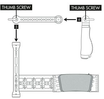
7. Loosen THUMB SCREWS to adjust HANDLES and ROSETTE ARMS to desired position
