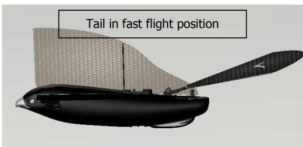
\* For outdoor flights, in a big space or for fast flights: adjust the tail in a low position (using the notch 1 or 2). Notch 2 is recommended for beginners. Notch 1 is for best performance but requires a bit of practice, and wings adjustment (see below).
