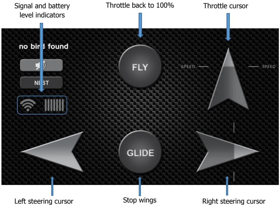
**EXPERT flight mode:** Using this mode, hold your smartphone in the horizontal position using both hands and manipulate the controls using your thumbs.
