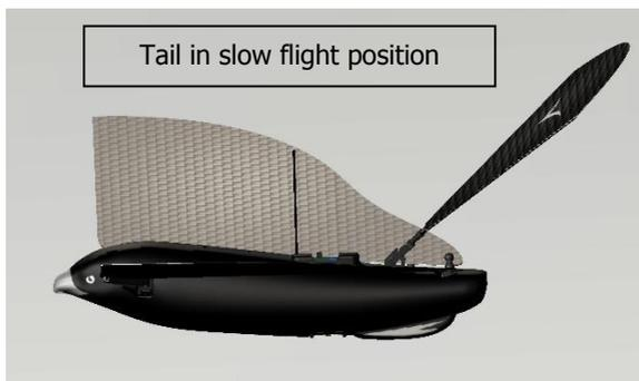
\* For indoor flights, in a confined space, or for slow flights: set the tail in a high position (choose the notch n° 3, starting from the bottom, among the 5 possible positions). The notches 4 and 5 are not recommended at begin.
