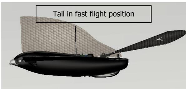
\* For outdoor flights, in a big space or for fast flights: adjust the tail in a low position (using the notch 1 or 2). Notch 2 is recommended for beginners. Notch 1 is for best performance but requires a bit of practice, and wings adjustment (see below).
