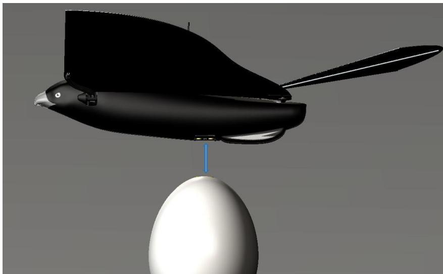
To charge BIONIC BIRD, simply connect the magnetic contact points situated under the bird's body and the top of the egg. They magnetically connect to each other automatically and the bird will sit firmly on the egg.
