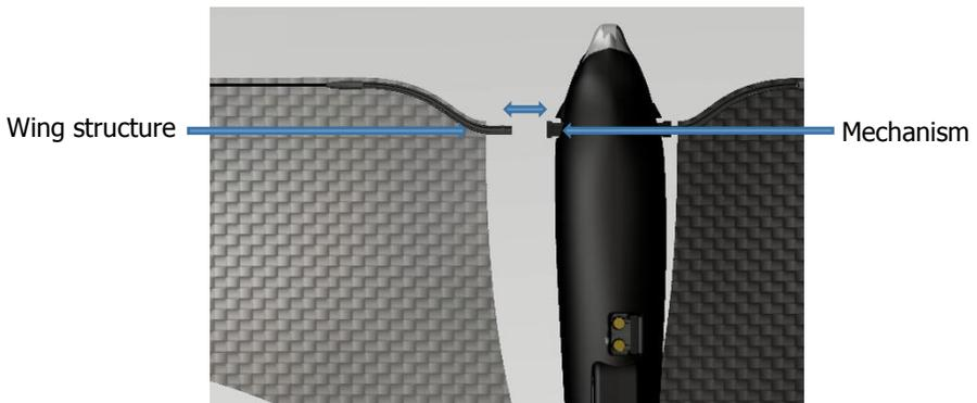
Then detach the front of the wing: hold the wing structure firmly and pull it out so that it comes out the slot. It is not necessary to change both wings, when just one is broken. Choose the appropriate spare wing (left or right) corresponding to the one to be replaced. Proceed reverse way: Start by inserting the wing structure in the slot, you should feel a "click" which means that the wing is correctly inserted. Clip the back of the wing to the round knob, underneath the tail.
