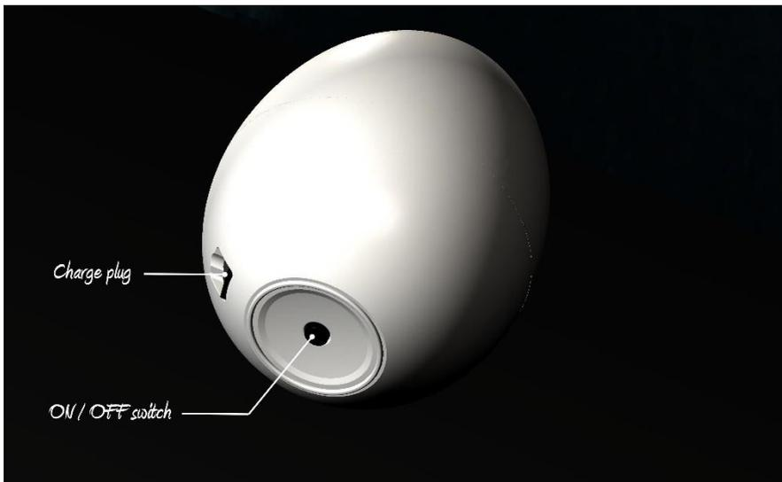
The first thing to do is to switch the egg ON, with the button located under its bottom. The bottom of the egg will lit blue. NB: If the egg doesn't lit, it may be discharged. You need to charge it again (see below).
