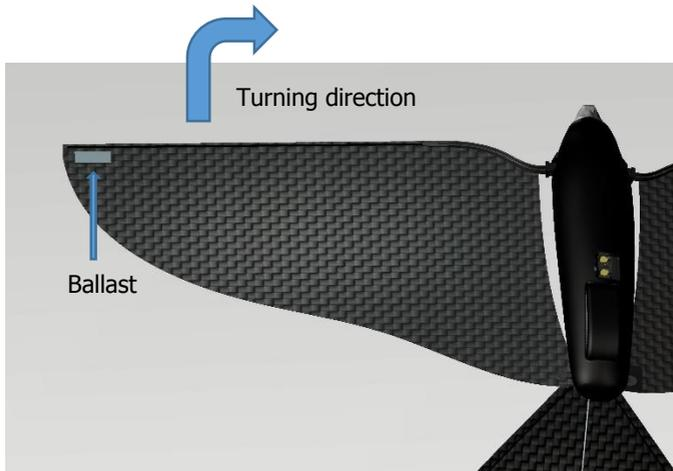
If the bird tends to turn to the right, add some weight to the left wing: Take one of the aluminium tape piece and stick it near the tip of the right wing, below the wing, as shown on the picture.
