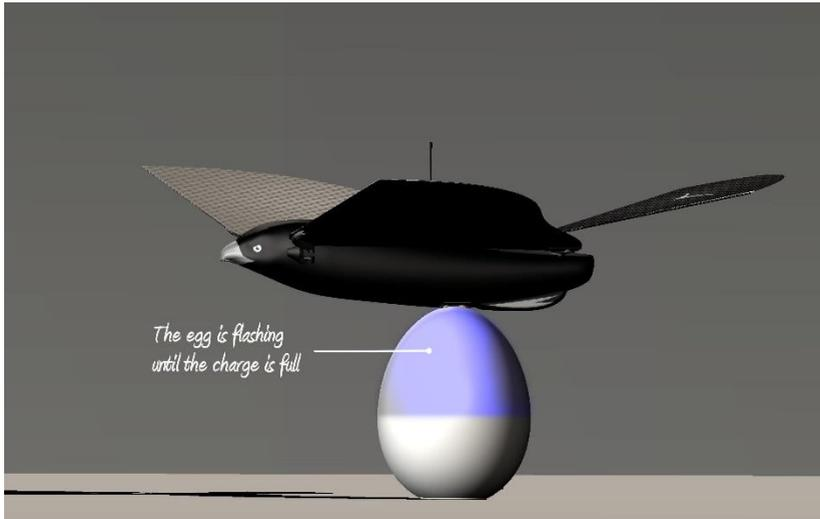
The upper part of the egg will start to blink when it starts to charge. Charging takes around 12 minutes. The egg will stop blinking and remain lit when BIONIC BIRD is fully charged and ready to fly again.
