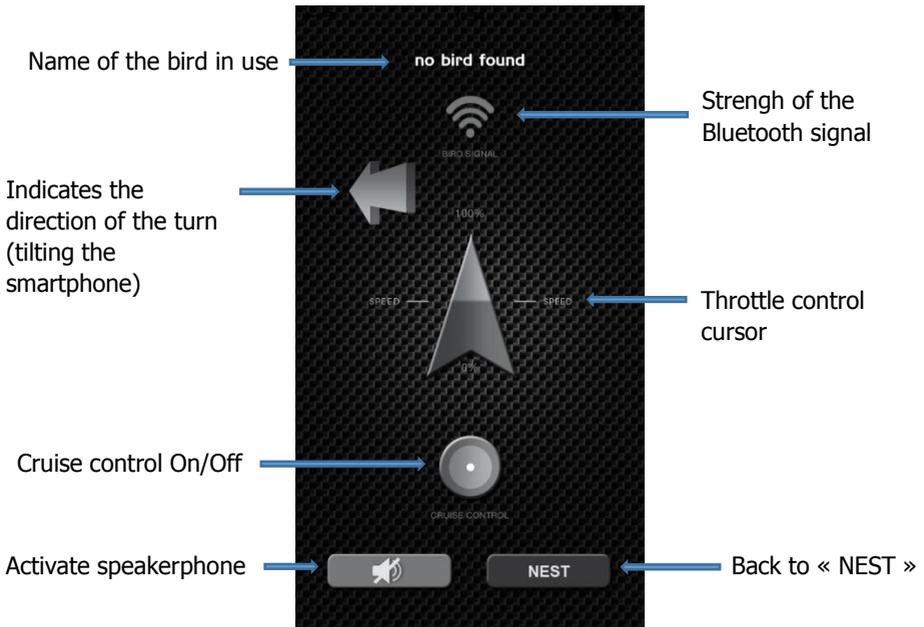
**EASY flight mode:** Using this mode, hold your smartphone with one hand, controlling the throttle cursor with your thumb, and tilting your device to control the flight direction.
