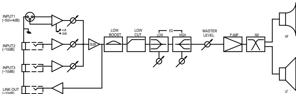
EQ Control.....LOW: ±3 dB at 60 Hz
