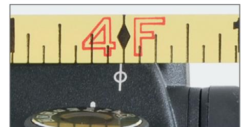
8. If the distance has changed, the flange focal distance of the lens must be adjusted by using the colored shims.
