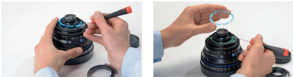
12. Place the black EF adapter ring on the lens barrel and tighten the screws using a torque of 0.4 Nm.
