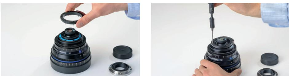
13. The next step is to place the silver EF mount on the EF adapter ring and tighten the screws using a torque of 0.4 Nm.
