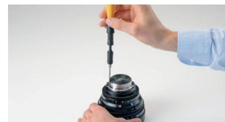
7. When the torx screws have been tightened, the lens can be fitted to a camera with a PL mount and used.
