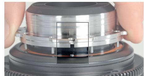
6. Tighten the eight torx screws with the T6 torque wrench using a torque of 0.4 Nm.
