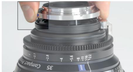
4. Please note the correct orientation of the Micro 4/3 and the E mount to the serial number on the lens barrel.
