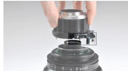
5. Tighten the torx screws using a torque of 0.4 Nm.
