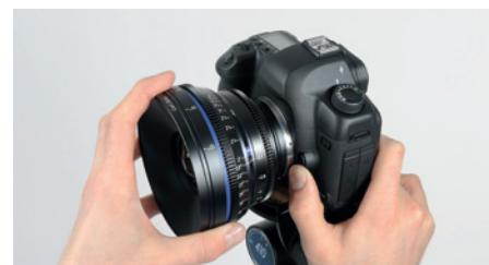
10. Remove the EF mount and EF adapter ring (cf. section C 2–4).
