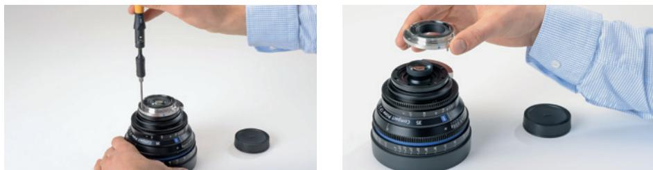
3. Remove the eight torx screws of the black EF adapter ring and place the ring and the screws on one side.
