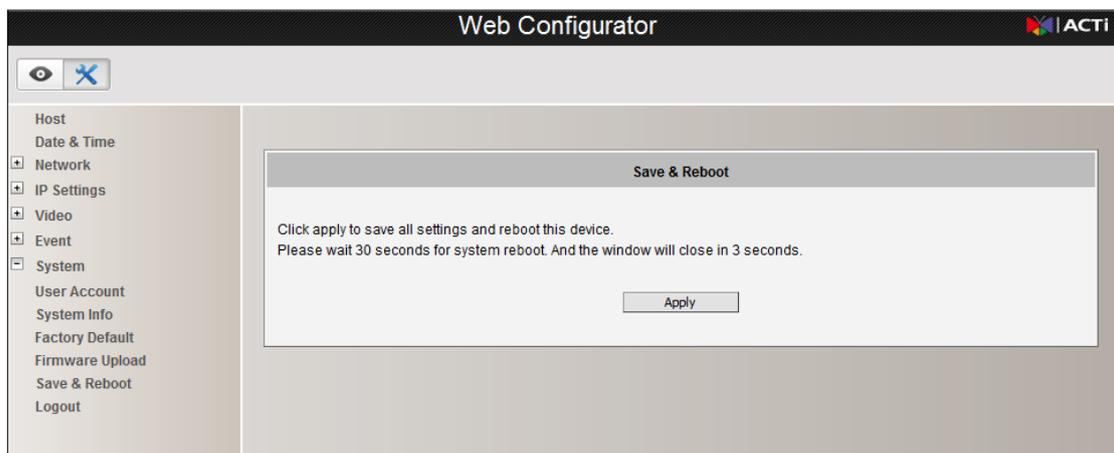
12. Wait for 30 seconds, and open IE again to connect to the **new IP**. (In this example, 192.168.0.101). For the second device or more you add into the network, please type the correct IP.
