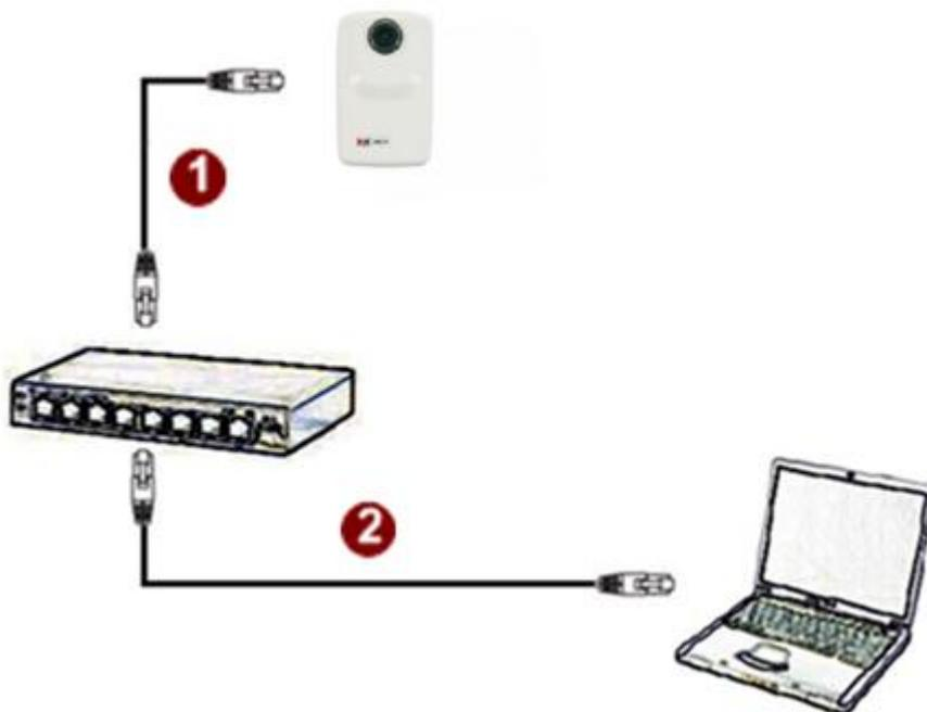
**Please use a PoE (Power over Ethernet) supported switch or injector:**
