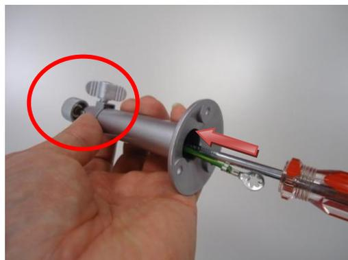
4. Connect another side of the ground wire with the hole of stand and use the screw to through them. Then, install on the wall or ceiling.
