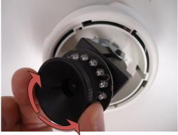
Remove the lens focus tuner.
