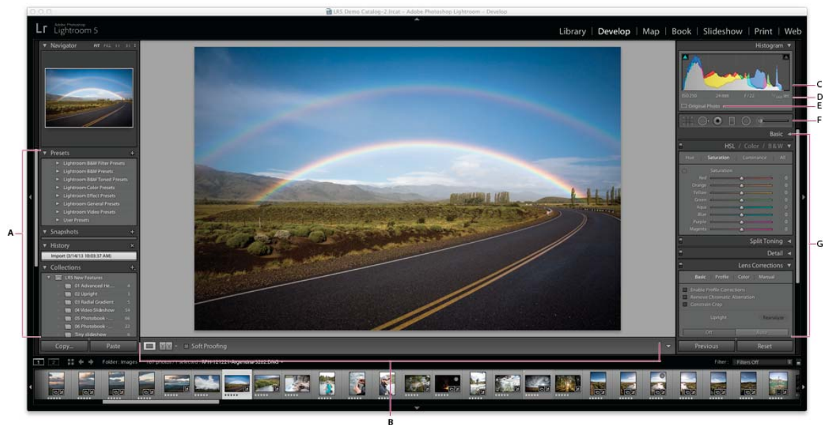
A Presets, Snapshots, History, and Collections panels B Toolbar C Histogram D Photo Information E Smart Preview status F Toolstrip G Adjustment panels
