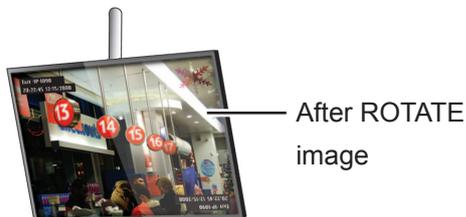
After executing ROTATE, touch the ▼ button again to rotate the picture back to its normal state.
