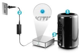
Turn on the computer, plug in the power adapter and connect the Thunderbolt cable to the computer.
