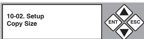
3. Press ENT to display the current configuration setting.
