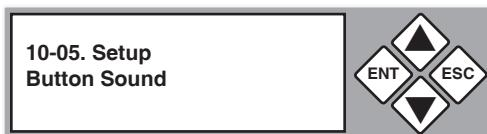
3. Press ENT to display the current configuration setting. The default is “On”.
