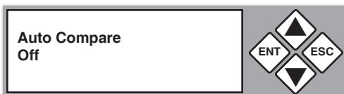
4. Use the arrow buttons ( $\blacktriangledown\blacktriangleup$ ) to modify the setting. After you change a setting, remember to press ENT to save it.
