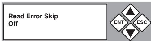
4. Press the arrow buttons (**▼** or **▲**) to toggle the option “On” or “Off”. After changing a setting, remember to press **ENT** to save it.
