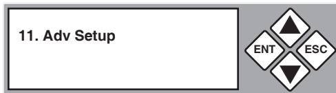
2. Use the arrow buttons (**▼** or **▲**) to scroll to “Read Error Skip”. The following screen will be displayed.
