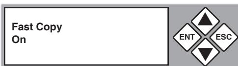
4. Use the arrow buttons ( $\blacktriangledown$ ,  $\blacktriangle$ ) to toggle between “On” and “Off”. Once you change a default, remember to press **ENT** to save it.
