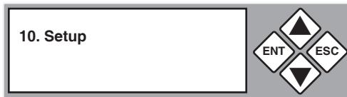
2. Use the arrow buttons ( $\blacktriangledown$ ,  $\blacktriangle$ ) to toggle between the subfunctions. Press ENT to select “Startup Menu”. The following screen will be displayed.
