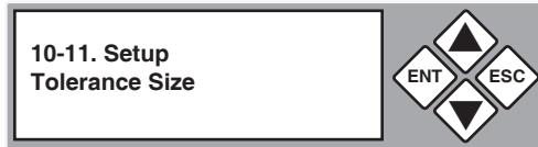
3. Press ENT to display the current configuration setting. (Off or 1 - 100%)
