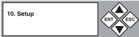
**Note:** After changing any of the configuration options, you must press ENT to accept the change. Once all changes are complete, press ESC to exit the Setup menu. The following screen will be displayed.
