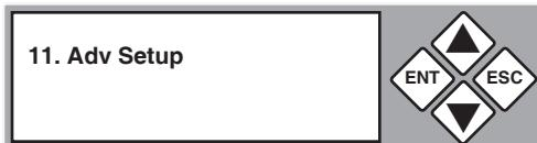
**Note:** After changing any of the configuration options, you must press **ENT** to accept the change. Once all changes are complete, press **ESC** to exit the Adv Setup menu. The following screen will be displayed.
