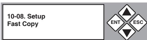
3. Press **ENT** to display the current configuration setting. The default is “On” (only used space will be copied).
