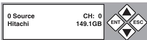
4. Use the arrow buttons ( $\blacktriangledown$  or  $\blacktriangle$ ) to show information about any additional hard drive that is connected. The following screen will be displayed.
