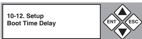
3. Press ENT to display the current configuration setting (0-99 sec).
