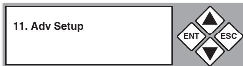
3. Use the arrow buttons (**▼▲**) to select “Update Firmware”, and then press **ENT**. The system will begin scanning for a new firmware version. If found, screens similar to the following will be displayed.
