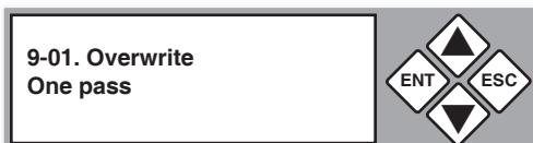
3. Use the arrow buttons to scroll between the types of overwrite: One Pass, 3 Pass, and 7 Pass.
