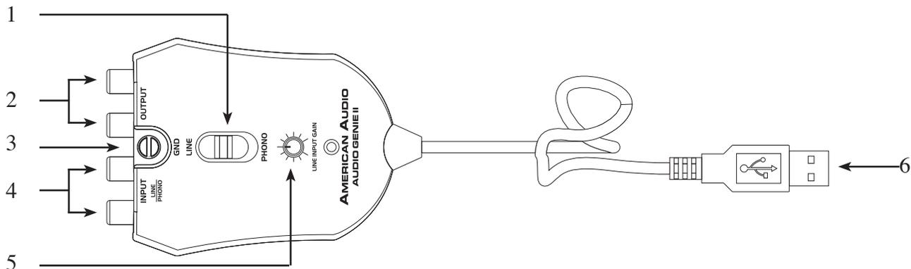
**1. Line In/Phono Switch** - This switch is used to select the input source assigned to the input jacks. The button must be in the “Phono” position for turntable operation.
