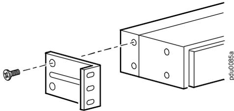
2. Install the PDU using hardware included with your rack or enclosure. The PDU will occupy one U-space.
