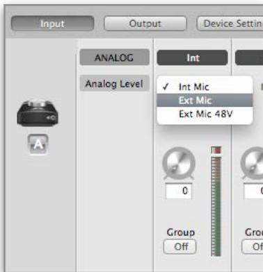
Select the Analog Level setting that corresponds to the microphone source you'd like to record. For example, if you have a microphone connected to the XLR connection on the breakout cable, select **Ext Mic** from the Analog Level menu on channel 1. If you would like to utilize ONE's built-in microphone, select **Int Mic**. Channel 2's source is always the 1/4" Instrument input.
