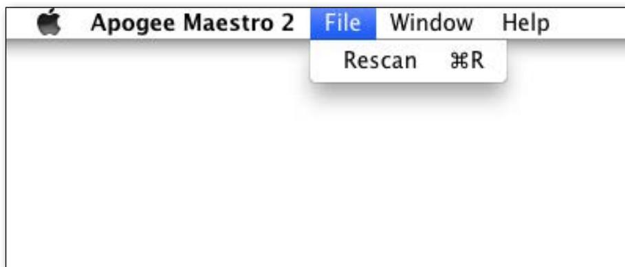
**Rescan** - Choose this menu item to re-initialize the link between Maestro software and Apogee hardware connected to the Mac in the case where the hardware is correctly connected and powered on but not detected in Maestro.
