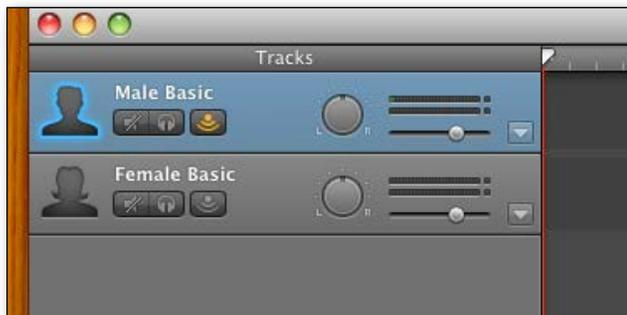
5. To hear input, click on the Monitoring button in the GarageBand track. If the button doesn't appear, choose **Track > Show Monitoring for Real Instrument Tracks**.
