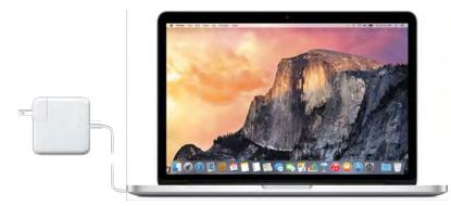
**Charge the battery.** Connect your MacBook Pro to a power outlet using the included cable and 60W MagSafe 2 Power Adapter. The battery recharges more quickly when the computer is off or in sleep.
