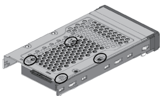
Figure 2-4-1. Installing 2.5-inch SAS/SATA Drive
