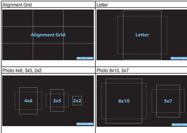
When QuickFit is activated, press the control buttons on the front panel to make adjustments. The QuickFit OSD displayed in the lower right corner of the screen will guide users to make selections.
