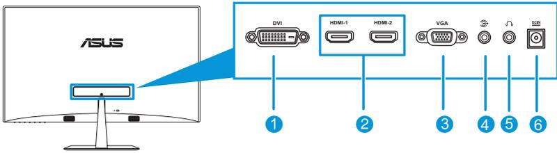
1. **DVI port** (Available for model VX238T and VX238N): This 24-pin port is for PC (Personal Computer) DVI-D digital signal connection.
