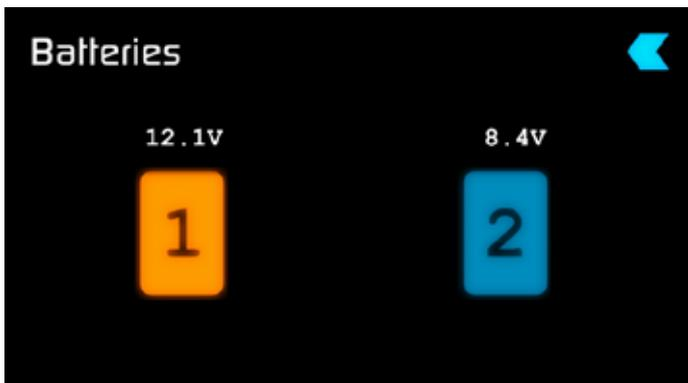
In the picture above we see Battery 1 is full and active and Battery 2 is currently inactive and 1/4 depleted. If no battery is present it will show an X in the picture and will be Black in colour as pictured right.
