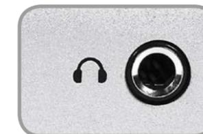
This can be used instead of or alongside speakers to get an idea how your mix sounds on headphones, or to provide artist headphone mix (or even to drive a small set of loudspeakers from an unbalanced Y-split cable).
