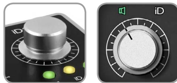
To mute an output, press the encoder quickly. If you only want it to mute momentarily then hold it down, and when it is released it will unmute the audio. In software, press the output icon to mute it.
