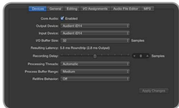
If you are using the iD mixer to monitor input signals while recording, be sure to disable Logic’s software monitoring to avoid phasing as the same source will be heard twice with a short delay between the low latency DSP signal and the delayed software monitoring signal.
