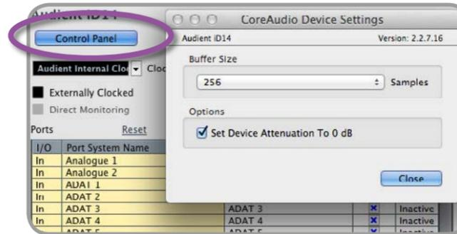
I/O ports can be renamed in the device panel such that they better represent what you connect to them (for example Main Monitors, Headphones). This is useful as any names chosen here will be those displayed when assigning i/o on track input/output channel routing.
