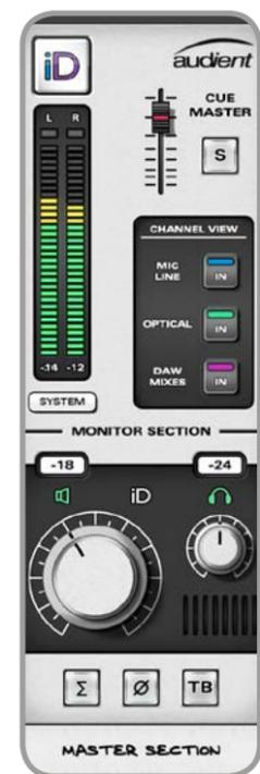
For simple monitoring / listening or in the box mixing it may be cleaner to view just the master section. When fully expanded via ADAT with a device like an ASP800, you can view all channels (after 10 mono slots, a scroll bar appears).
