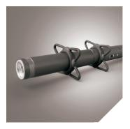
To accelerate switching of microphones, remove the microphone and the suspenders as a unit from the shock mount. Obtain extra pairs of suspenders and leave them on the microphones. To change microphones, carefully peel the suspenders away from the shock mount to free the microphone. Slide the new microphone into place and carefully stretch the suspenders over the retainers.
