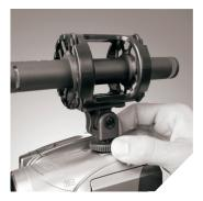
The Auray DUSM-1 Shock Mount features a shoe adapter for camera mounting. Insert the microphone into the Shock Mount before mounting onto the camera. Slide the shoe adapter into the accessory shoe and tighten the thumbwheel. Do not overtighten.
