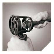
Insert the XLR lead end of the microphone into the opening of the shock mount. Continue pushing the microphone through the second of the shock mount suspenders. Rotate the microphone so that any controls are accessible, and leave room for any windscreens you plan to use.
