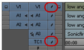
Sync Lock icon (top) and Sync Lock All button (bottom) in the Track Selector panel
