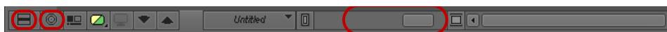
Left to right: Timeline Fast Menu button, Focus button, and scale bar in the Timeline bottom toolbar
