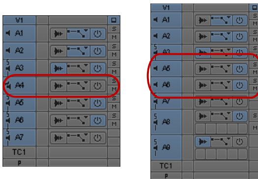
Stereo track A4 (left) split into mono tracks A4 and A5 (right)
