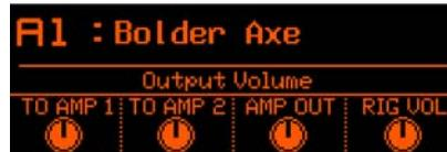
This mode offers fast access to the output settings for the current Rig. It provides four lit control knobs. These are labeled TO AMP 1 (Output To Amp 1 volume), TO AMP 2 (Output To Amp 2 volume), AMP OUT (amp output volume), and RIG VOL (Rig output volume).
