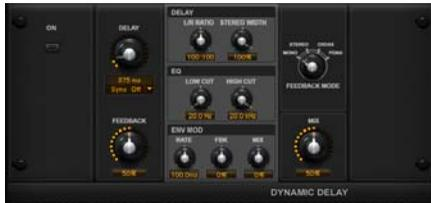
This stereo delay effect is based on the Air Dynamic Delay plug-in that comes with Avid's Pro Tools recording software. A powerful effect, Dyn delay can be synchronized to Rig or Session tempo, and offers an envelope follower, that lets you modulate various parameters, based on the amplitude envelope of incoming signal. This effect includes the following controls:
