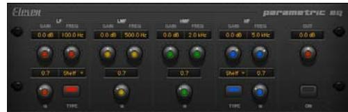
This effect provides a high-quality 4-band EQ, with adjustable gain, frequency, Q (bandwidth), and output for each band. The Low and High bands let you switch between the following functions:
