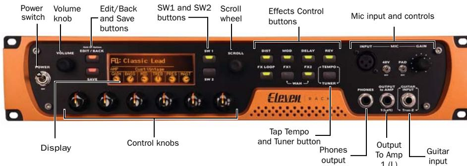
Figure 1. Eleven Rack front panel
