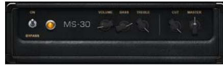
The MS-30 amp model is based on a US-made, early-90s boutique combo amp, the first design by its manufacturer. Featuring a 30-watt EL84-based power section and two twelve-inch speakers in an open-back configuration, it excels at a range of sounds, from squeaky-clean all the way to beautifully-overdrive high-gain tones.
