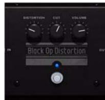
Inspired by an 80s-era op-amp-based distortion pedal, BlackOp Distortion offers massive crunch and power. Its hard-clipping drive can squeeze aggressive rhythm and lead tones out of soft-sounding vintage amps, and create surprisingly hard-edged tones when paired with more modern amps.
