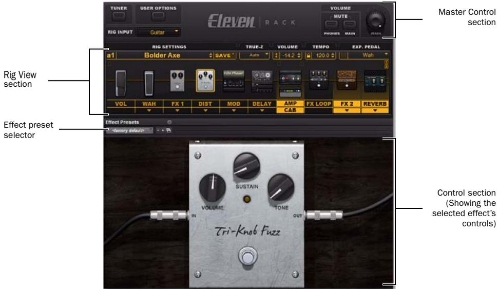
Figure 10. Eleven Rack Control window (in Pro Tools)
