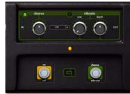
Based on a heavyweight late-70s analog chorus/vibrato pedal, CI Chorus/Vibrato offers warm, liquid modulation effects. In Chorus mode, the signal is routed through a modulated short delay, which is mixed with the dry signal, creating a washy, doubled sound.
