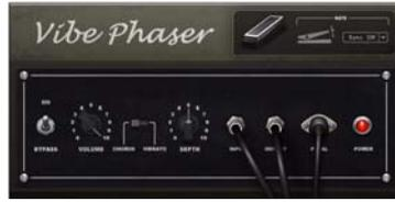
The psychedelic-era phaser that inspired our Vibe Phaser effect was traditionally paired with an expression pedal that could be used to vary the rate of pitch modulation over time. Like the C1, you can choose to run it as a Chorus, with the modulated and dry signals mixed together, or in Vibrato mode, which leaves the pitch-modulated signal alone, with rippling, disorienting effects.
