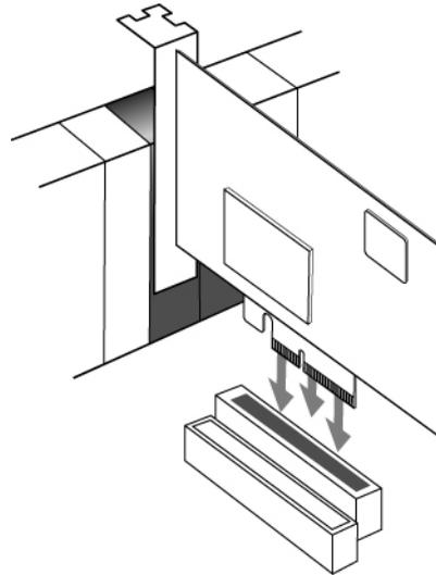
*Inserting the Pro Tools|HD Native card into a PCIe slot*
