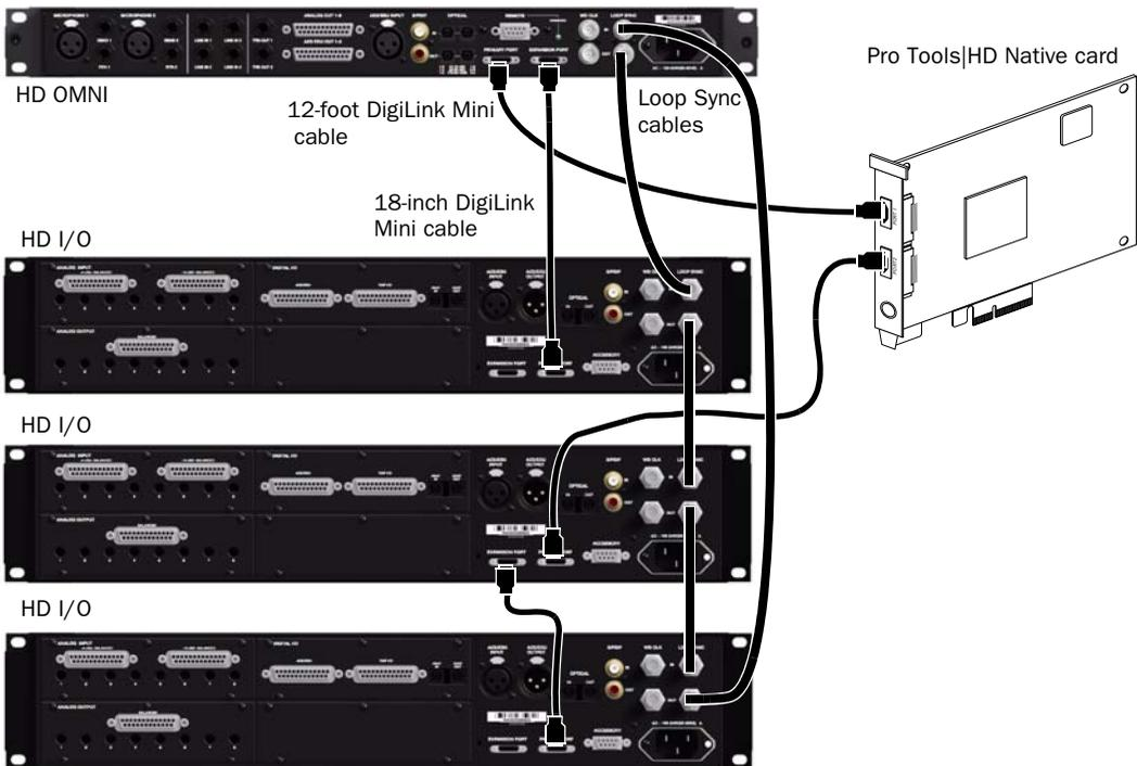
Figure 2. Making DigiLink Mini and Loop Sync connections
