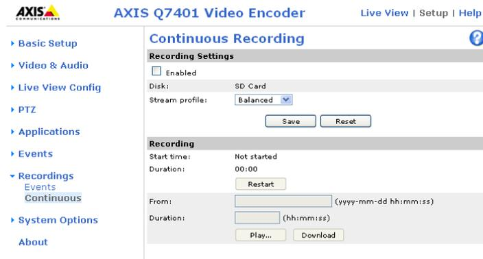
The AXIS Q7401 video encoder can be configured to continuously save video to local storage. Automatic Disk Cleanup should be enabled when using Continuous Recording to prevent the local storage from becoming full. See *Storage - Disk Management*, on page 42.
