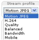
The Stream Profile drop-down list allows you to select a customized or pre-programmed stream profile on the Live View page. Stream profiles are configured under **Video & Audio > Stream Profiles**, see *Stream Profiles*, on page 14 for more information.
