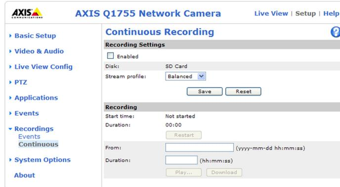
The AXIS Q17 Series Network Camera can be configured to continuously save video to local storage. Automatic Disk Cleanup should be enabled when using Continuous Recording to prevent the local storage from becoming full. See *Storage - Disk Management*, on page 42.
