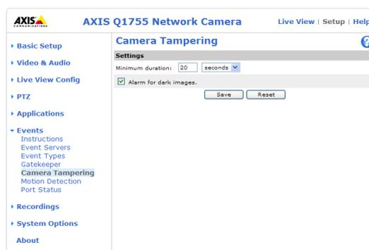
If the camera lens is sprayed or covered so that the camera live view becomes dark, it will not be possible to distinguish this situation from other situations where the same effect is seen, such as when lighting conditions change.
