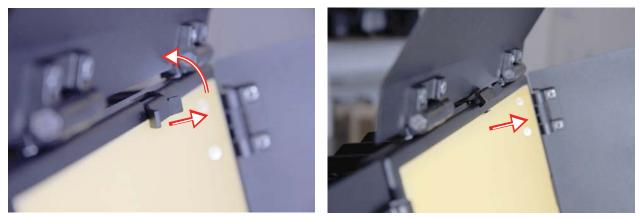
Pull the lock out and up, so that it rests on the top. This will push the media a little out.
