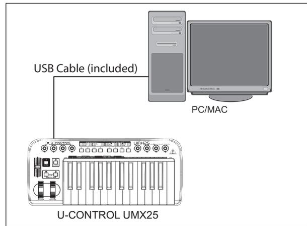
Fig. 1.1: Power supply via USB
