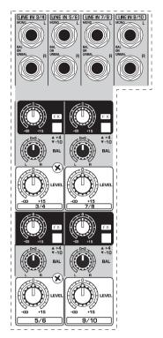
Fig. 2.2: Connectors and controls on the stereo channels
