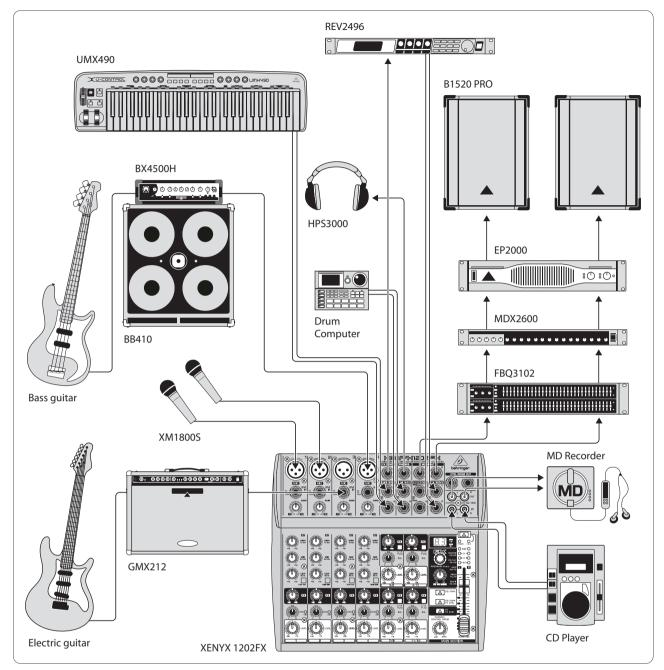
Fig. 3.2: Live application of the 1202FX
