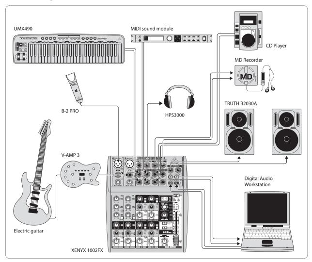
Fig. 3.1: The 1002FX in a recording studio
