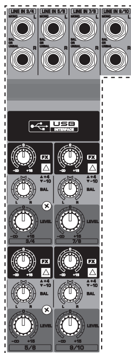
Fig. 2.2: Connectors and controls on the stereo channels
