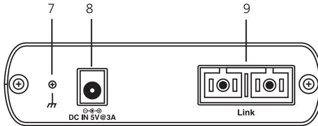
Figure 2-4. Back panel of the remote unit.
