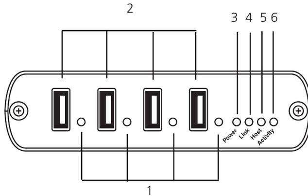
Figure 2-3. Front panel of the remote unit.
