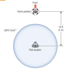
**CAUTION:** Starting the motors sets the home location. The quadcopter must be approximately 16 feet (5 meters) from where the pilot will stand during flight, pointing away from the pilot. If the aircraft is pointed in any other direction, the SAFE Circle TM feature will not function as expected and may result in personal injury or damage to property. Once the aircraft's motors are started, do not change your position.
