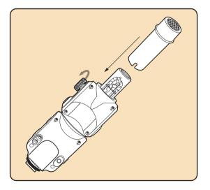
Make sure to properly tighten the bare-bulb flash's accessory port to secure the snoot.
