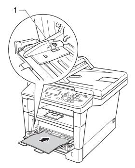
4 Lift up the support flap to prevent paper from sliding off the face-down output tray, or remove each page as soon as it comes out of the machine.
