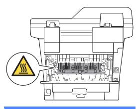
5 Pull the green tabs at the left and right hand sides toward you and fold down the fuser cover (1).
