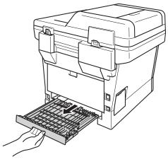
Pull the jammed paper out of the 7) machine or out of the duplex tray.
