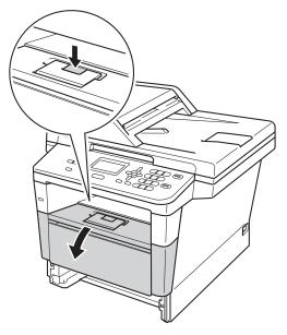
5 Slowly take out the drum unit and toner cartridge assembly. The jammed paper may be pulled out with the drum unit and toner cartridge assembly, or this may release the paper so you can pull it out from inside of the machine.
