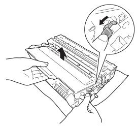
7 Put the toner cartridge back into the drum unit until you hear it lock into place. If you put the cartridge in correctly, the green lock lever will lift automatically.
