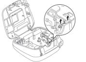
2. Install a new cutter unit. Push it in until it snaps into place.
