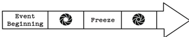
2. **Sleeping:** In Multi Shot, LV5 will send a Shutter Close Signal at Event End. During the Freeze period after shutter closes, LV5 ignores all Event happening. The Freeze setting does not affect the length of shutter signal.
