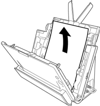
**7 Close the front unit by gently pushing it up on both sides until it clicks into place. Make sure that the front unit is completely closed by pushing until you hear a click.**
