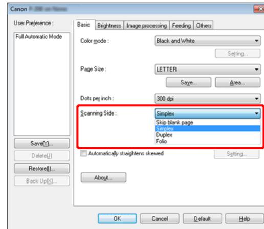
If [Skip Blank Page] is selected, the [Setting] button is enabled, and you can adjust the level for judging whether pages are blank.
