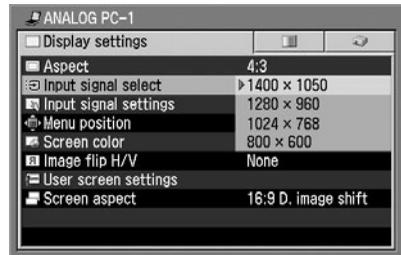
Select an input signal type suitable for the computer from the displayed signal types. Press the [MENU] button when you finish.
