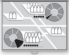
Select this to project a computer screen with aspect ratio of 4:3 (SXGA+ [1400 by 1050 dots] or XGA [1024 by 768 dots]). If you select this mode to project the computer screen with aspect ratio of 5:4 (SXGA [1280 by 1024 dots]), it is compressed vertically or horizontally.
