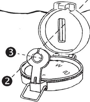
3. Without moving the compass, glance down through the lensatic magnifier and read the bearing from the compass card.
