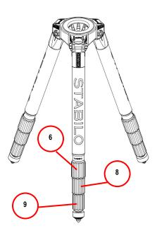
4 - Repeat point 3) to open the second and the third **CARTONI STABILO** stages operating the medium (8) and the lower (9) knob and raise the **CARTONI STABILO** height
