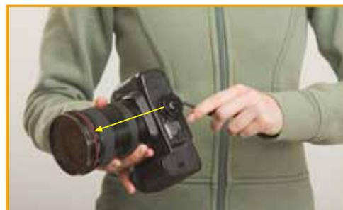
2. Attach the Camera Hub by threading it into the 1/4" tripod mount of your camera with the Allen Key. **MAKE SURE IT IS REALLY TIGHT!** Check frequently!
