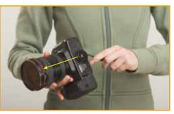
Attach the Camera Hub by threading it into the 1/4" tripod mount of your camera with the Allen Key. MAKE SURE IT IS REALLY TIGHT! Check frequently!
