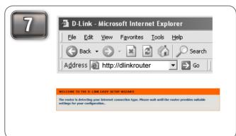
From the computer you connected the router to, open a web browser and enter http://192.168.0.1 or http://dlinkrouter. Press Enter and you will be directed to the D-Link Setup Wizard page, which will detect your Internet connection type. Follow the on-screen instructions to configure your Internet settings. After setting up your router, you will be given the option to create a mydlink account. Go to www. mydlink.com and enter your acount information.
