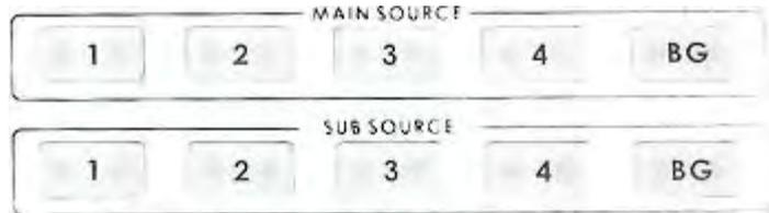
The source you select (by pressing one of the buttons; a bright red LED on the selected button lights for confirmation) on the Main Source bus is what is sent to the Video output. This means that you can perform cuts between sources by simply pressing different buttons.
