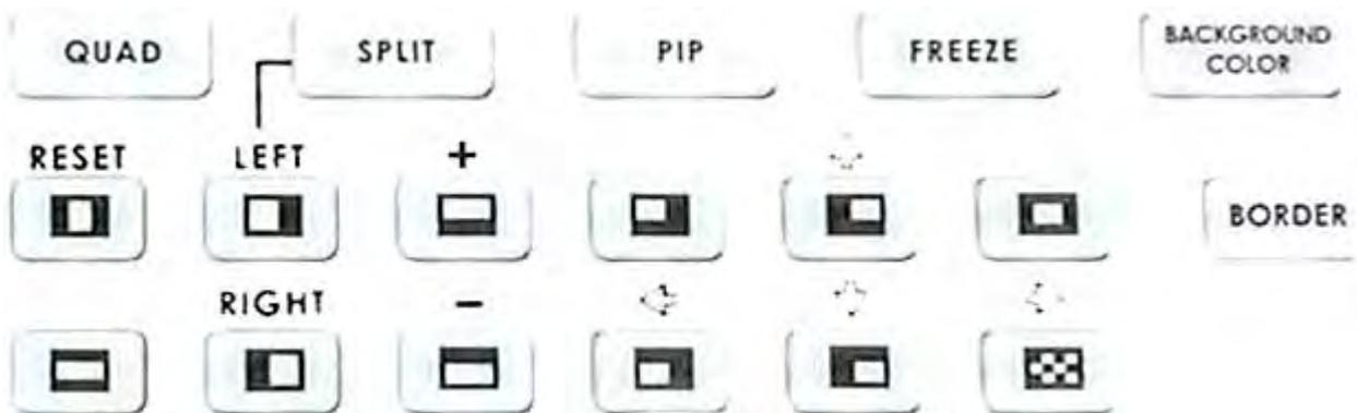
In the Video Effects section, try the Quad effect (5.). Press the button to engage the effect; the LED will light. You can see 4 input sources showing on the program monitor at the same time.
