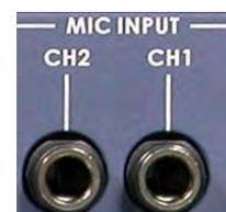
7. **MIC CH1:** When a stereo 1/4" jack is connected to CH1 only, the CH1 and CH2 **Faders** (page 13) will have equal volume on each channel. When both CH1 and CH2 have a MIC connected, each fader channel will adjust the respective input from the rear panel.
