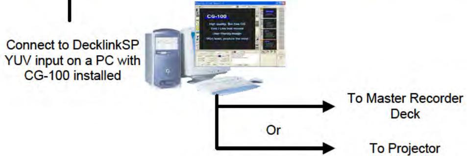
Using YUV output (with a breakout cable) on SE-500 to communicate with a PC with Decklink SP CG overlay card and CG-100 CG software (page 42) to perform a text overlay for the output video.
