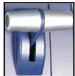
If no transition is selected, moving the T-Bar performs a fade between the selected sources.
