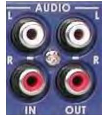
9. **Audio Output:** A RCA stereo line level analog audio output, carrying the signal present at the output of the audio mixer section (see **Controls and Operations**, page 20).
